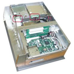
3. Unscrew the screws of the FDD and CD-ROM module and take off the FDD and CD-ROM.
